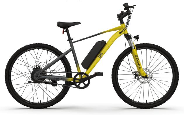
Frame : 18" High Tensile Steel Frame
