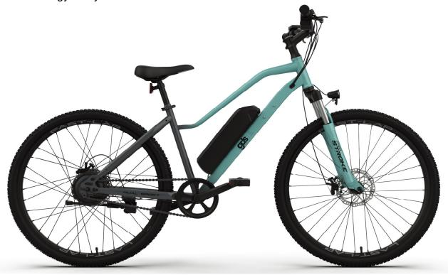
Frame : 18" High Tensile Steel Frame
